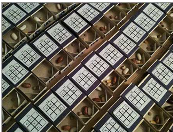
Figura 8: MENACE (Matchbox Educable Noughts and Crosses Engine)
