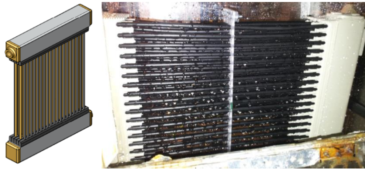
Figure 2. Falling-film air-solution contactor
