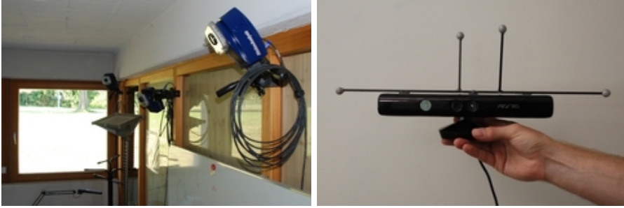
Figure 2.8: Motion capture system used in the TUM RGB-D dataset [92]. Left 1 : multiple cameras mounted on the wall pointed at the measuring zone. Right 1 : Kinect depth camera with reflective markers. By tracking the markers seen by the cameras, the pose of the sensor can be retrieved.
