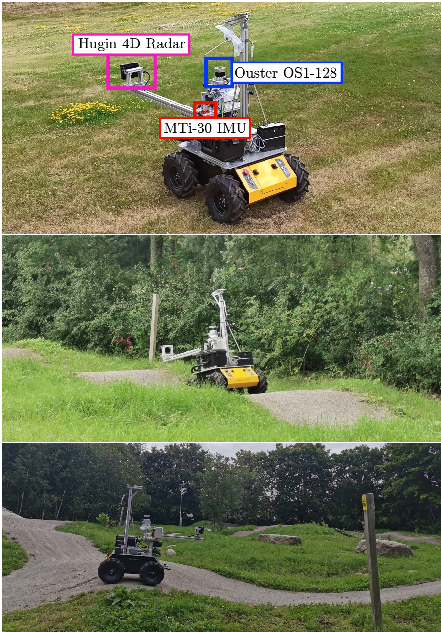
Figure 5.3: Sensor setup (top) and test environment from sequence 04 (middle and bottom).
