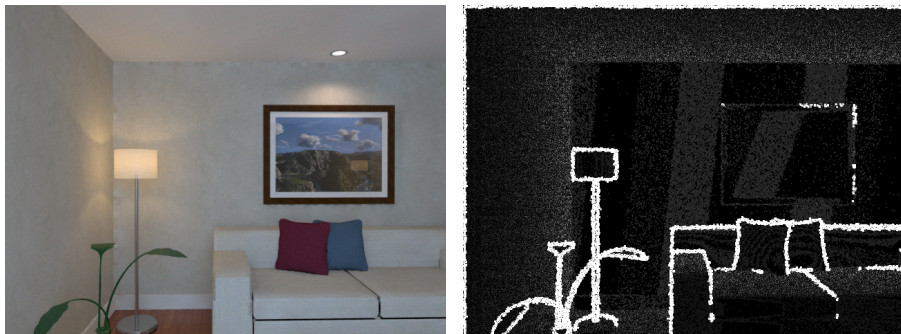
Figure 3.3: Image of a scene (left) and its corresponding flatness image (right). Light pixels represent areas in which the scene cannot be represented as a plane, examples of this being the edges of the objects.
