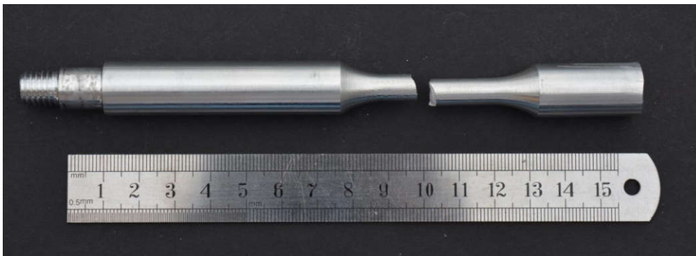
Figure 11. Rotating bar bending test fractured.
