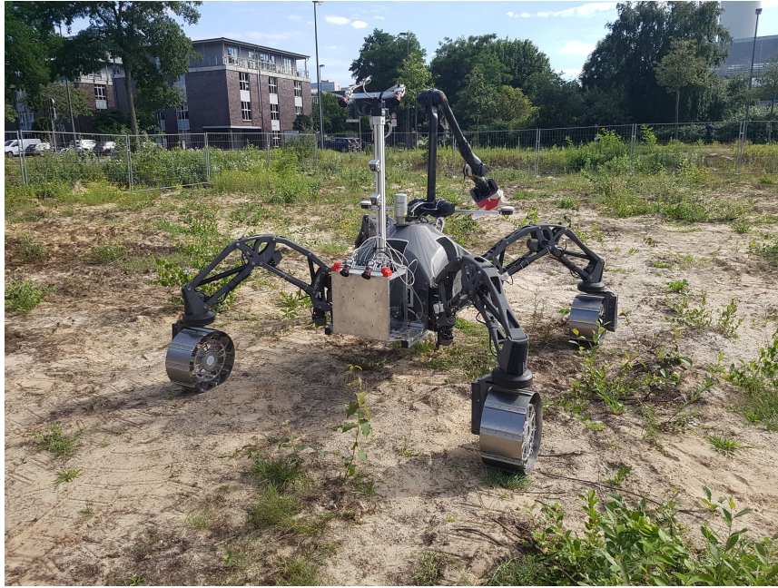
FIGURE 1.6: SherpaTT rover of DFKI during the H2020 ADE project.
