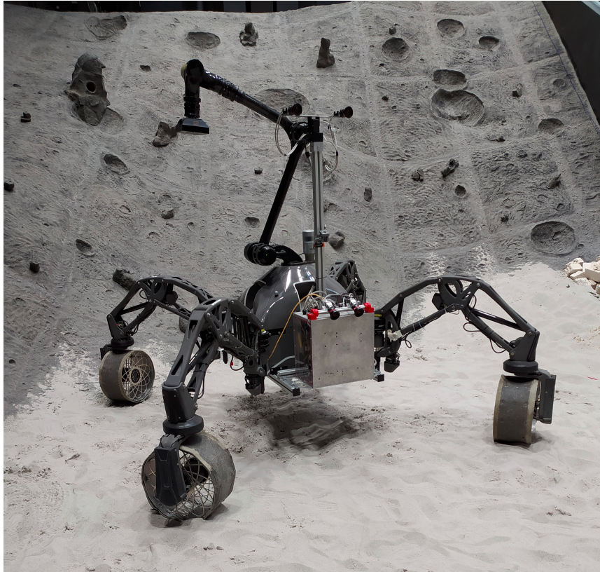
FIGURE 6.6: SherpaTT rover in the Lunar crater of the SpaceHall at DFKI RIC, Bremen.
