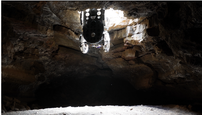
(a) CoyoteIII vertically descending through the skylight (DFKI RIC).
