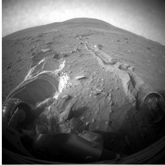
FIGURE 2.3: Wheels of the NASA Spirit rover sinking in loose Martian soil due to high slippage (NASA/JPL-Caltech).
