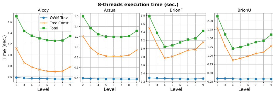
Figure 3.10: Optimization O3: tree construction, OWM traversal and total times depending on lev using 8 threads.
