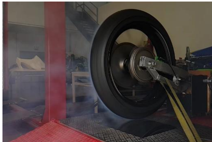
Figure A2. Burnout due to excessive slippage without TCS.
