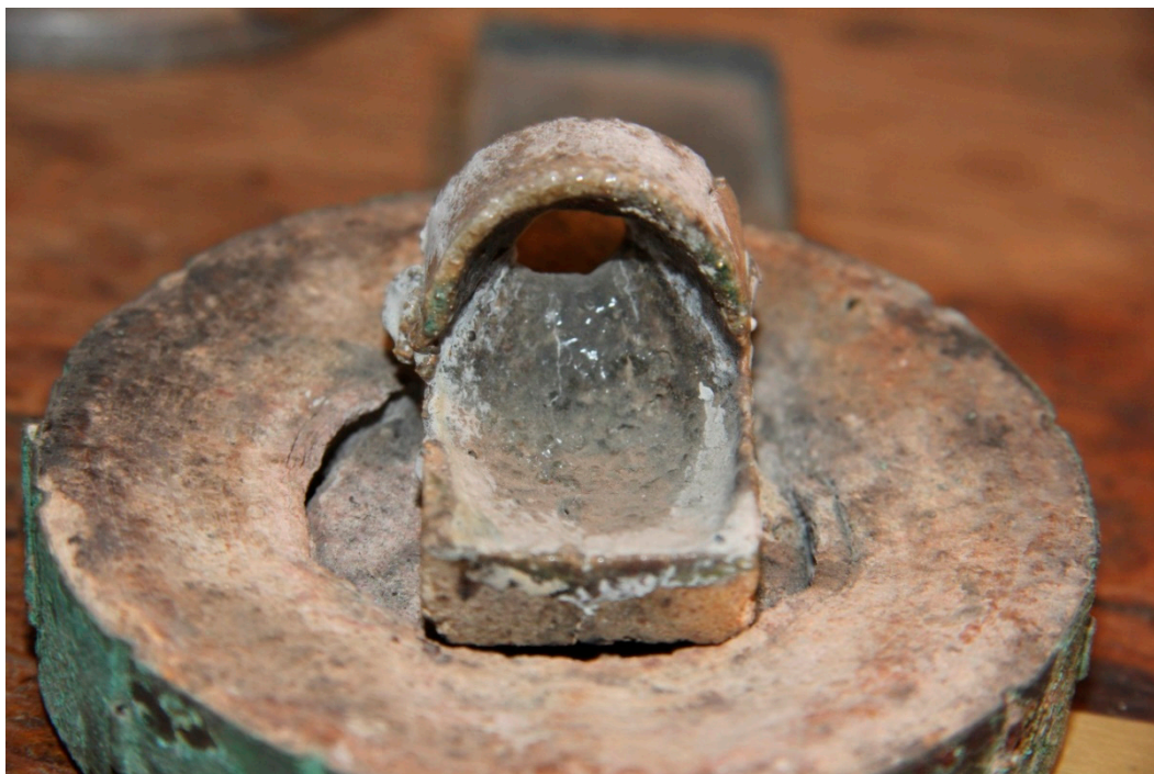
Figure 3. Crucible for melting metals that would be later inserted into a Solbrig-Platshick casting cylinder. Source: Dental Museum. Faculty of Dentistry. University of Granada (2021).
