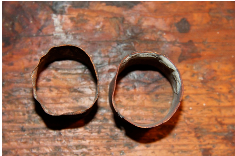
Figure 2. Asbestos liner inside casting cylinder. Source: Dental Museum. Faculty of Dentistry. University of Granada (2021).
