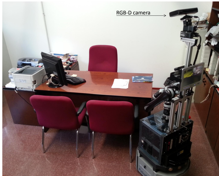
Figure 6: The mobile robot Rhodon gathering 3D data within an office room.
