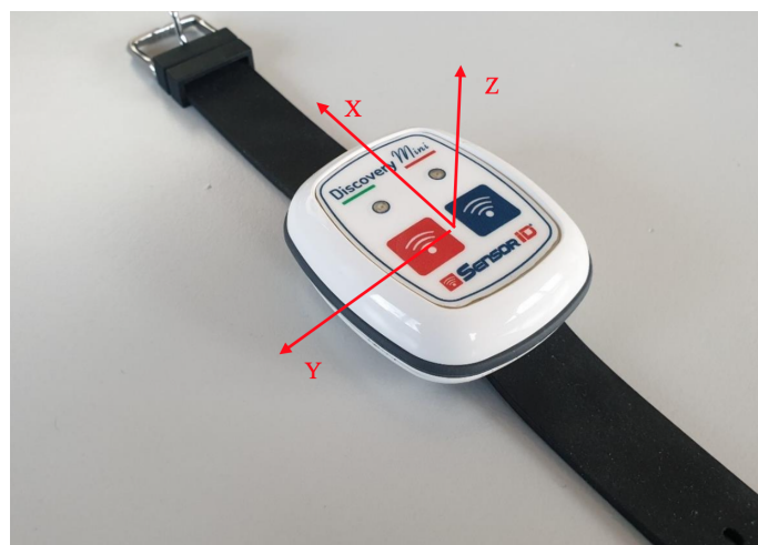
Figure 4. The Discovery Mini inertial sensor, showing the 3-axes.
