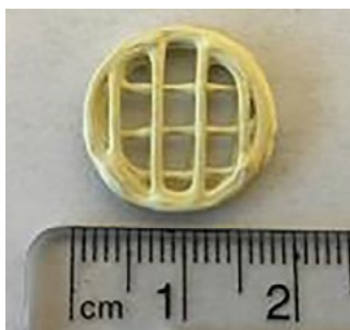
Figure 11. Torlon-zeolite monolith prepared by Thakkar et al. (2018)
