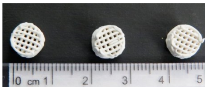
Figure 9. 3D printed zeolite monoliths prepared by Thakkar et al. (2016).
