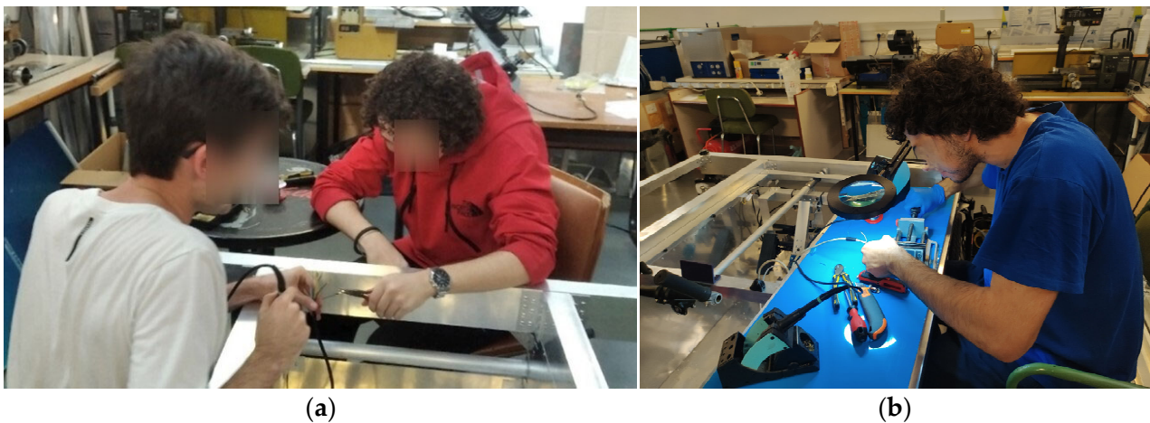
Figure 5. Electrical system manufacture. (a) Soldering; (b) Crimping.
