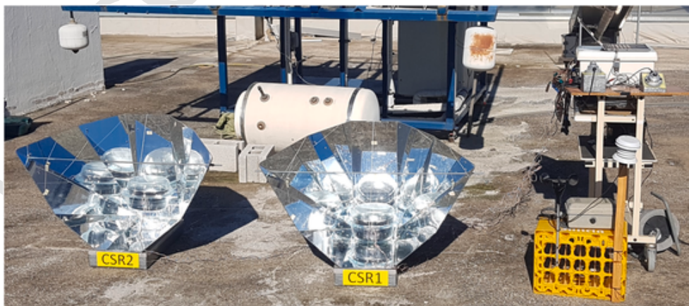
Fig. 2. Solar cookers CSR1 and CSR2 being tested, respectively, without and a trivet.
