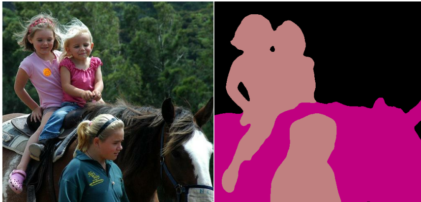
Figure 2.15: Semantic segmentation example from Deeplab (Chen et al. (2018)). As can be observed, the three people share the same mask as they are in the same class.
