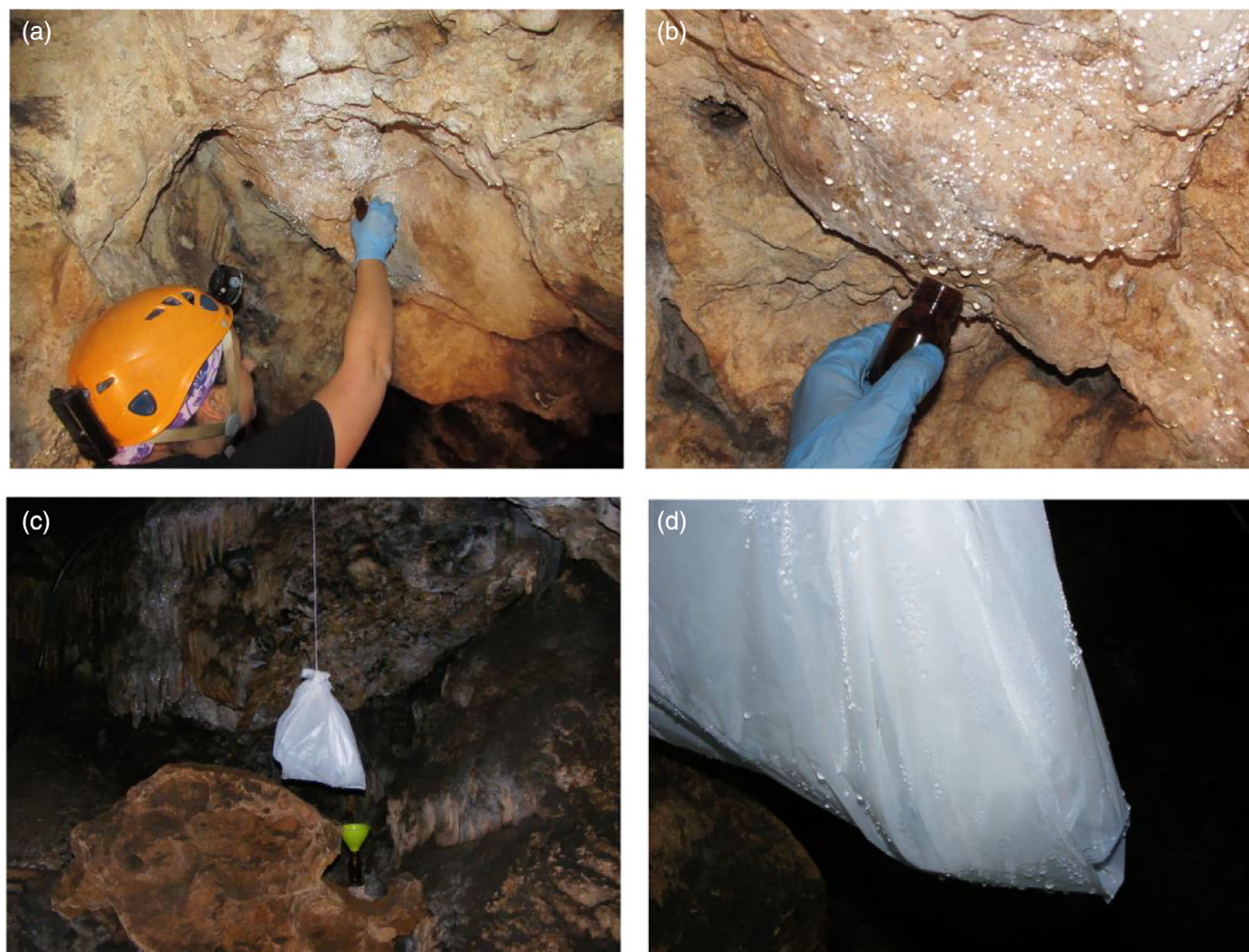
FIGURE 2 (a) Sampling of natural condensation water (Nw) in the ceiling of the area C2. (b) Detailed photo of the sampling method. (c) Device for sampling induced condensation water (Iw) in the area C3 and (d) detailed photo of water condensed on the ice bag
