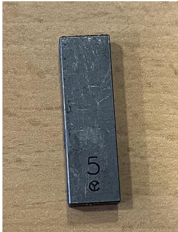
Figure 7. One of the gauge blocks used
