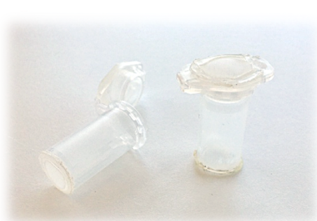
Figure 2.0.8: Test cylinder (modified Eppendorf) where A. swirskii females from each of the isofemale lines were isolated individually.
