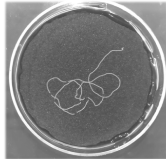
Figure 2.0.7: Processed image recorded by the robot from an A. swirskii individual path tracked during 1 min.
