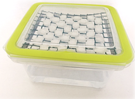
Figure 2.0.9: Desiccation chamber where test cylinders were placed. Each chamber had a different relative humidity (35, 50, 65%).
