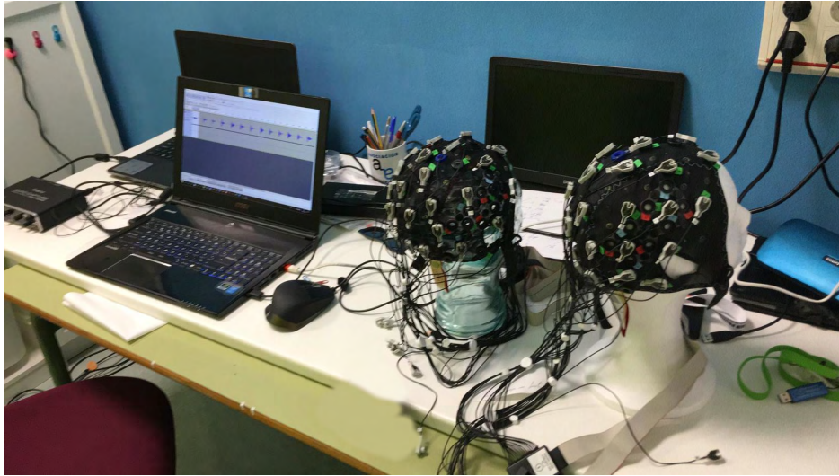
Figure 5.2: Laboratory view. actiCAP headset and NIRS acquisition systems
