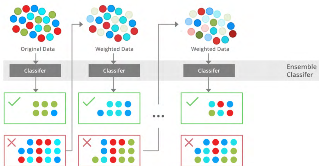
Figure 4.6: Illustration of a boosting ensemble. Each new classifier tries to correct the errors in the previous one [70]
