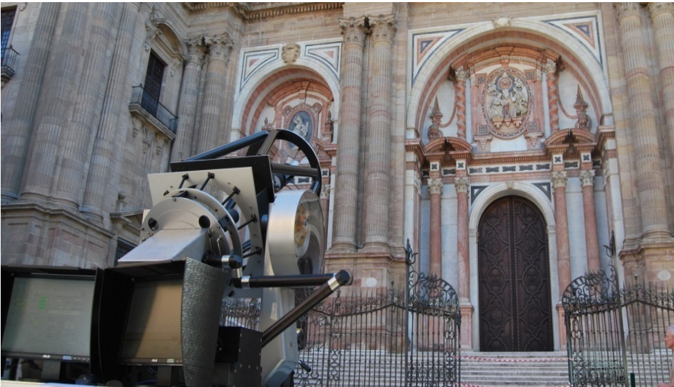
Fig. 1. Descriptive scheme on the working scenario. The emplacement of the LIBS platform, and section investigated, are highlighted.
