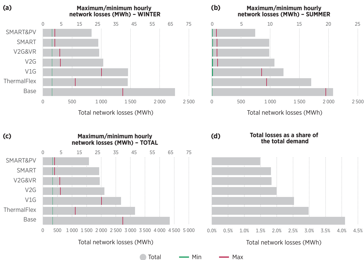
FIGURE 11 | Energy grid losses in (a) winter, (b) summer, (c) total and (d) total as a share of demand
