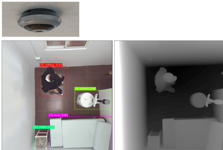
Fig. 9. (Top) The 360° Panoramic Indoor Fisheye Camera with 6MP SHD from ReoLink; and (Bottom) a rectified capture of the bedroom and the associated depth map.
