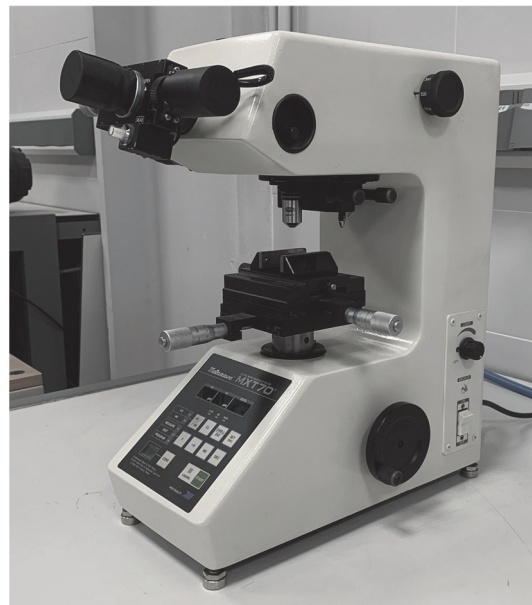
Figure 2. Micro-indentation tester Matsuzawa MXT70 used for Vickers microhardness.
