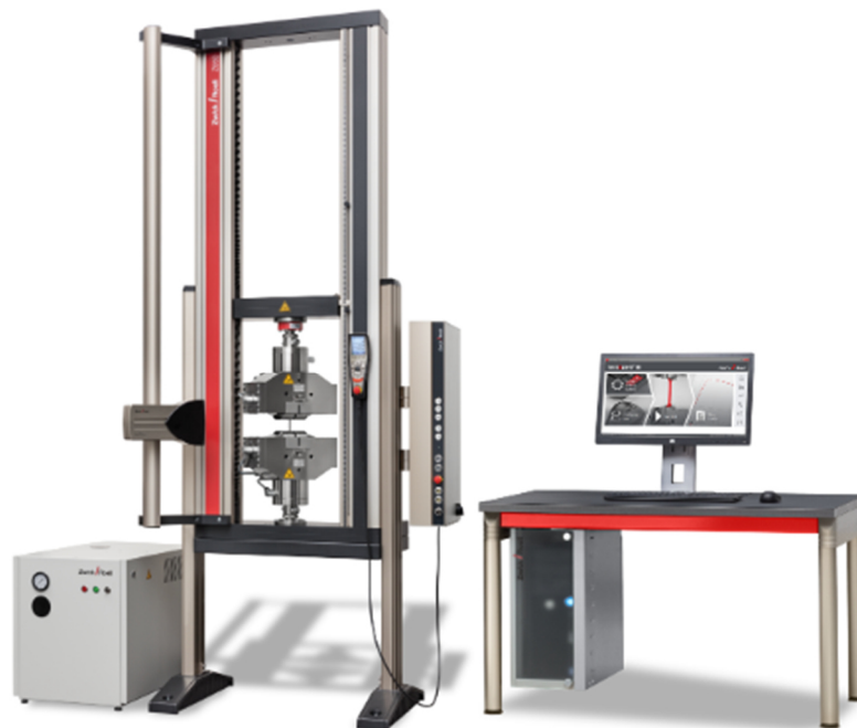
Figure 2.17. Uniaxial testing machine available at the Institute of Orthopaedic Research and Biomechanics of the University of Ulm and used for the load-to-failure tests performed.
