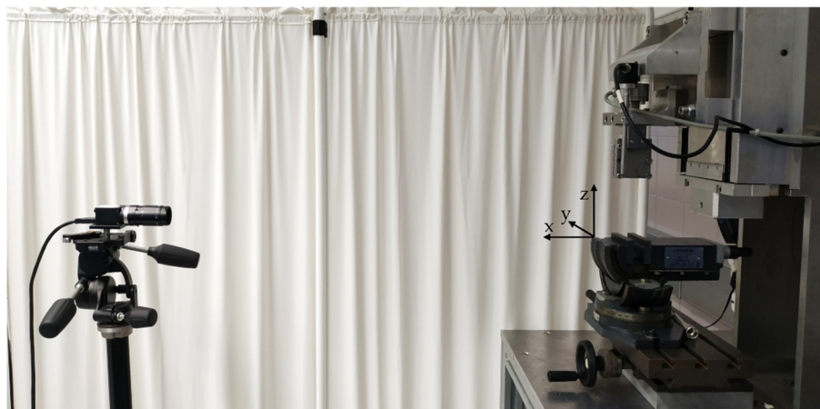
Figure 3.2. Uniaxial testing machine and videogrammetric system, with the Z axis corresponding to the traction direction and the ZY plane parallel to the image plane.
