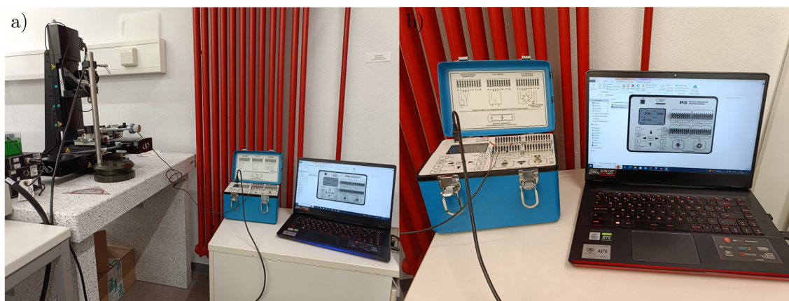
Figure 6.4. Setup prepared for recording the traction force induced by the suture using the traction device while the indentation test: a) multi-axial mechanical tester with the traction device connected to the strain indicator and recorder; b) strain indicator and recorder connected to the computer.
