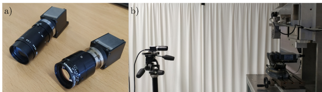
Figure 2.19. Devices used in the videogrammetric system in BIOCLINA. a) Digital camera with the PENTAX lens; b) Digital camera mounted in the tripod oriented to the uniaxial testing machine.
