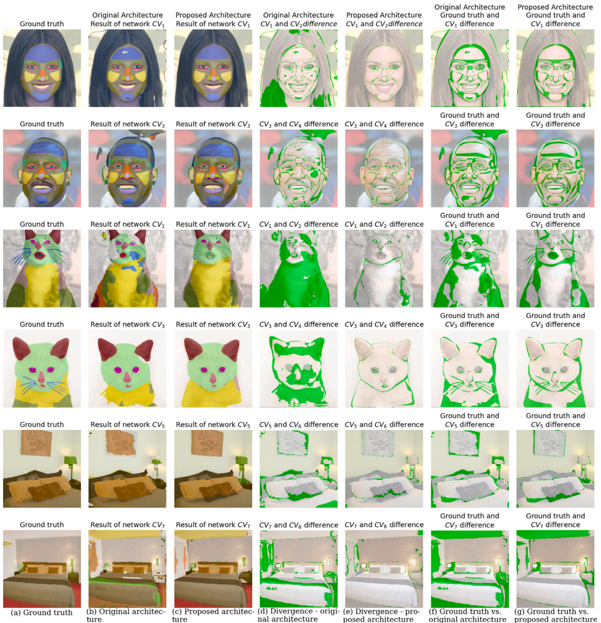
Fig. 7. Examples of the qualitative improvements observed in the Face, Cat, and Bedroom datasets: (a) ground truth segmentation; (b) segmentation resulted from the original DatasetGAN architecture; (c) segmentation resulted from the proposed architecture; (d) difference between the two cross-validation networks within the same fold for the original DatasetGAN and the proposed architectures; (e) difference between the two cross-validation networks within the same fold for the proposed architecture; (f) difference between the ground truth segmentation and the original DatasetGAN architecture; (g) difference between the ground truth segmentation and the proposed architecture.
