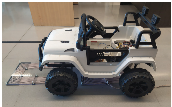
FIGURE 10 Implemented prototype for DWPT.
