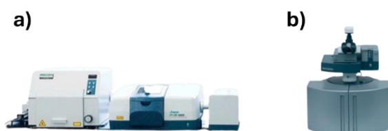
Figure 2.6. a) FT-Raman Jasco RFT-6000 and b) Bruker Micro-Raman Senterra.
