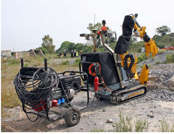
Fig. 1. The tracked mobile manipulator Alacrane (right) and its trailer (left) during an emergency response exercise.
