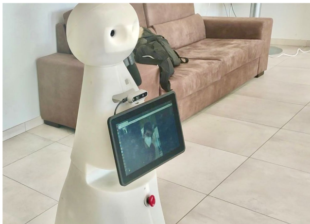
FIGURE 15 | CLARC robot during a videocall test, where the tablet shows the image of the family member on call.
