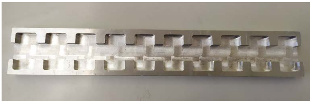
Figure 5.2: Aluminum cavity mechanized to fabricate the array.
