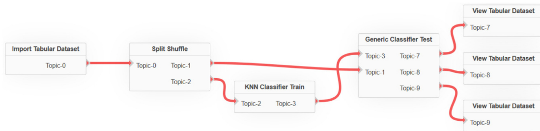
Figure 3.5: The Iris dataset classification workflow as visualized in the graphical tool. The initial step involves loading the dataset, followed by the second step, partitioning the data into training and testing sets. The training data is used to build a machine-learning model in the third step. The fourth step employs the trained model and the testing data to evaluate the classifier’s predictive performance. Ultimately, key metrics generated from the model are highlighted.
