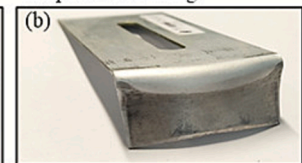
Incipient Wrinkling: iw W_0=54, l_0=20
