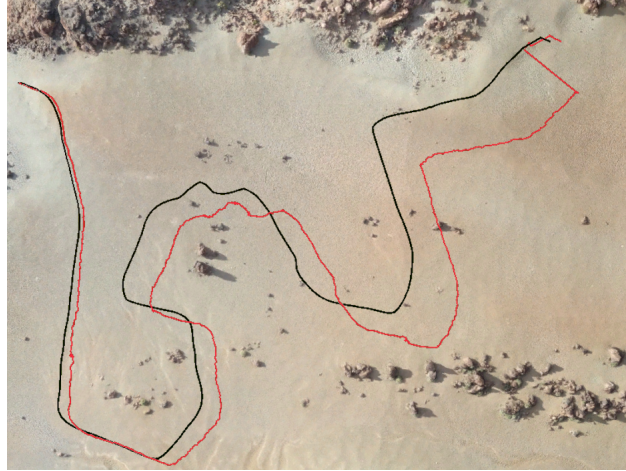
Figure 12: Orthographic views of the environment and the rover's traverses in it. The black and red colors correspond to the ground truth and SLAM paths accordingly. The pose correction is visible in the end of the traverse.
