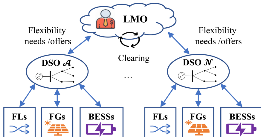
Figure 3.2: General diagram of the relationships between the stakeholders of the LEM formulation.
