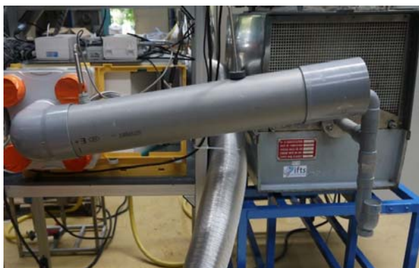
a) view of extraction duct
