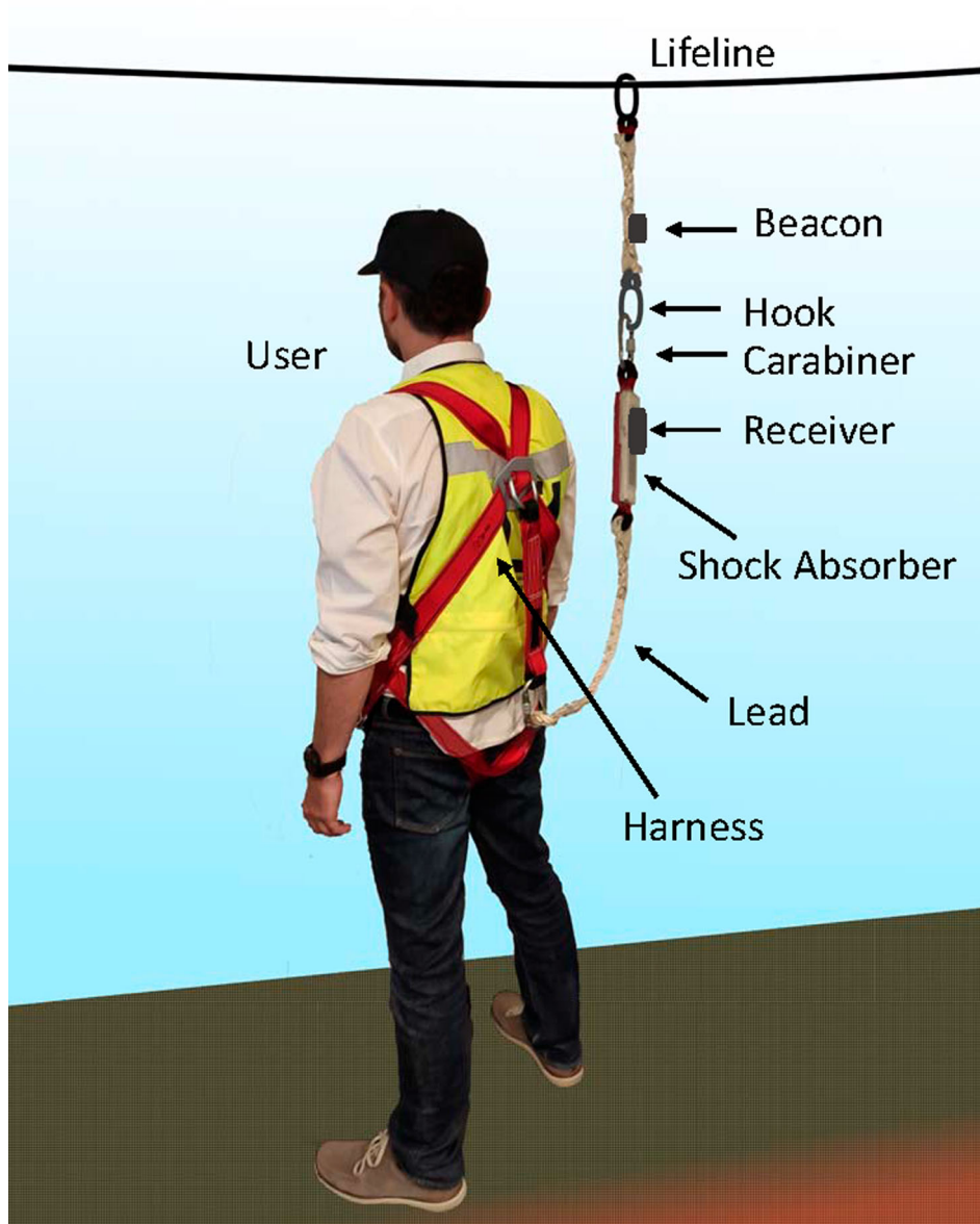
Figure 1. Harness with a Bluetooth Low Energy receiver and lifeline beacon system.
