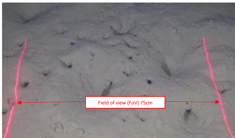
Figure 3.5: FU 30 Sample Image with laser lights showing the field of view
