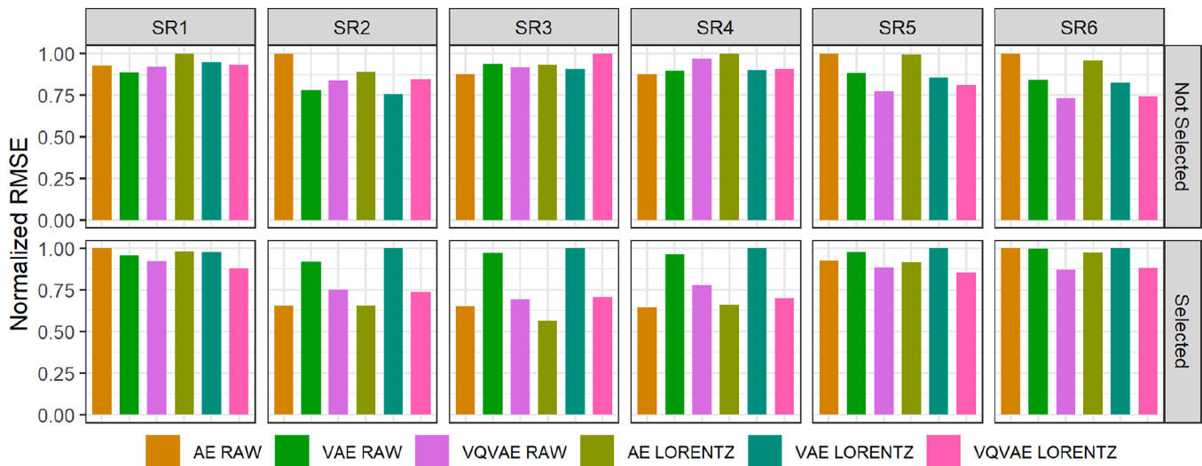
Fig. 6. RMSE normalized by the maximum value of each mode and type. Selected refers to the registers that present good condition to perform a LCF procedure.
