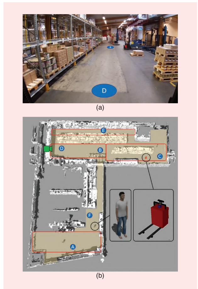
FIGURE 8. Real and simulated warehouse environments used during the experiments. (a) A picture from the real Orkla Foods warehouse. (b) A 3D model of the Orkla warehouse used in the simulation and a digital model of the small pallet truck. The robot deployment area is in orange, the goal locations are marked with blue circles, the pedestrian navigation areas are marked with red rectangles, and the camera location for the picture seen in (a) is marked with the green camera icon.
