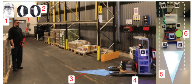
FIGURE 4. (1) The eye-tracker device. (2) The Empatica E4 band used for measuring electrodermal activity. (3) The SAR projection "arrow" projected on the shared floor space to convey the robot's navigation intent. (4) The robot (one of ILIAD's retrofitted AGVs) with the SAR intention communication system. (5) The defined AOI. (6) The eye gaze fixation.
