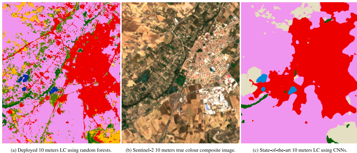
Fig. 1. 1(a), 1(b) and 1(c) present a comparative analysis of a specific region in Cintruénigo, Spain. While the LC classes may vary between the approaches, both demonstrate the presence of built-up areas (red) and cropland (pink). Notably, the state-of-the-art LC model exhibits characteristics of object-based classification despite the spatial resolution of 10 m. In contrast, the model using our methodology, leverages a pixel-based classification approach, enabling a higher level of detail in LC classification across any given area.
