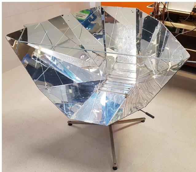
Fig. 3. Funnel cooker assembled to the tripod with stand to hold the cooking set.
