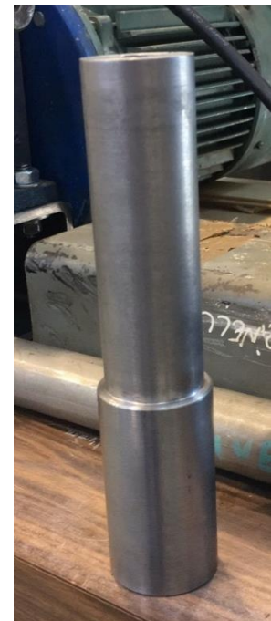
Fig. 5. Left - Sketch of the shaft and spindle anchored part; Right - shaft transmission part made of steel.
