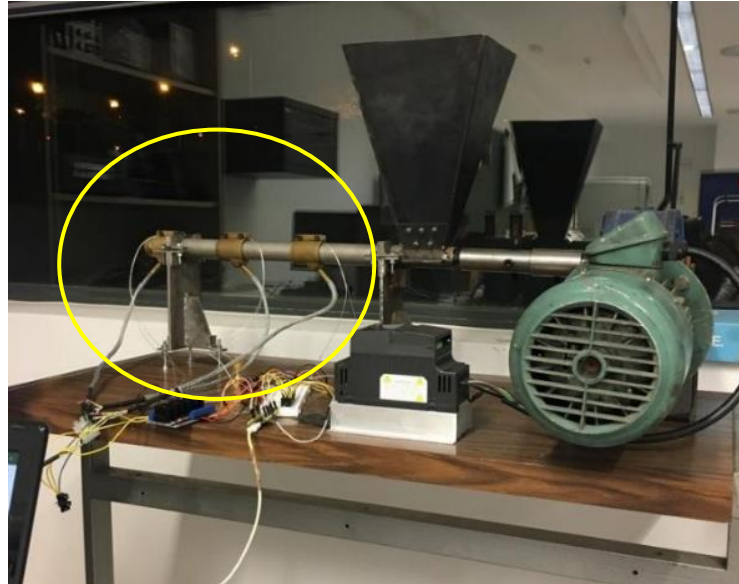
Fig.SU- 7. Resistors on MAREA Plastic's extruder
