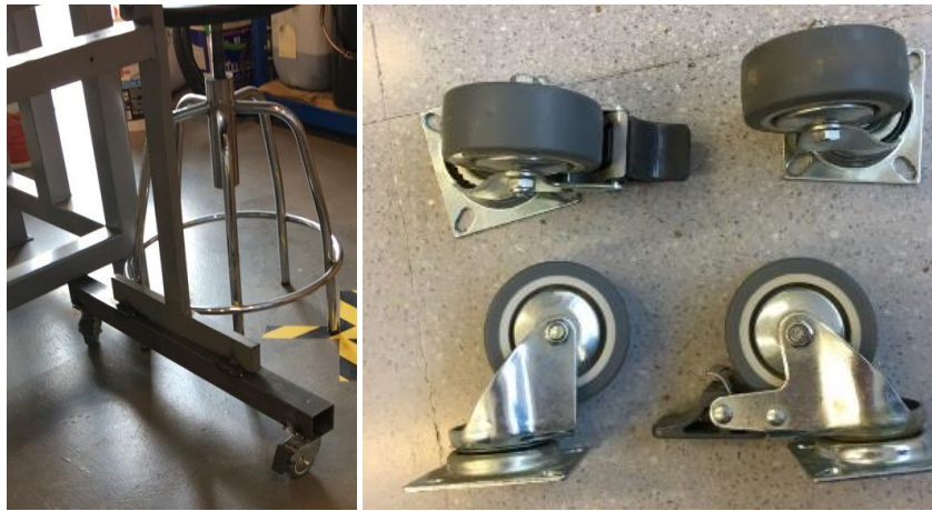
Fig.SU- 2 Welded reinforcement + wheels employed on the recycled table
