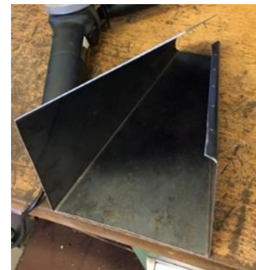
Fig. 4 Hopper design. Left - surface alignment on a sheet (Step 1); right - cutting and bending of the sheet (Step 2).
