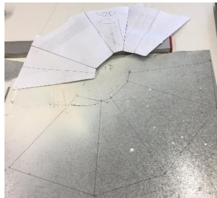
Fig. 4 Hopper design. Left - surface alignment on a sheet (Step 1); right - cutting and bending of the sheet (Step 2).
