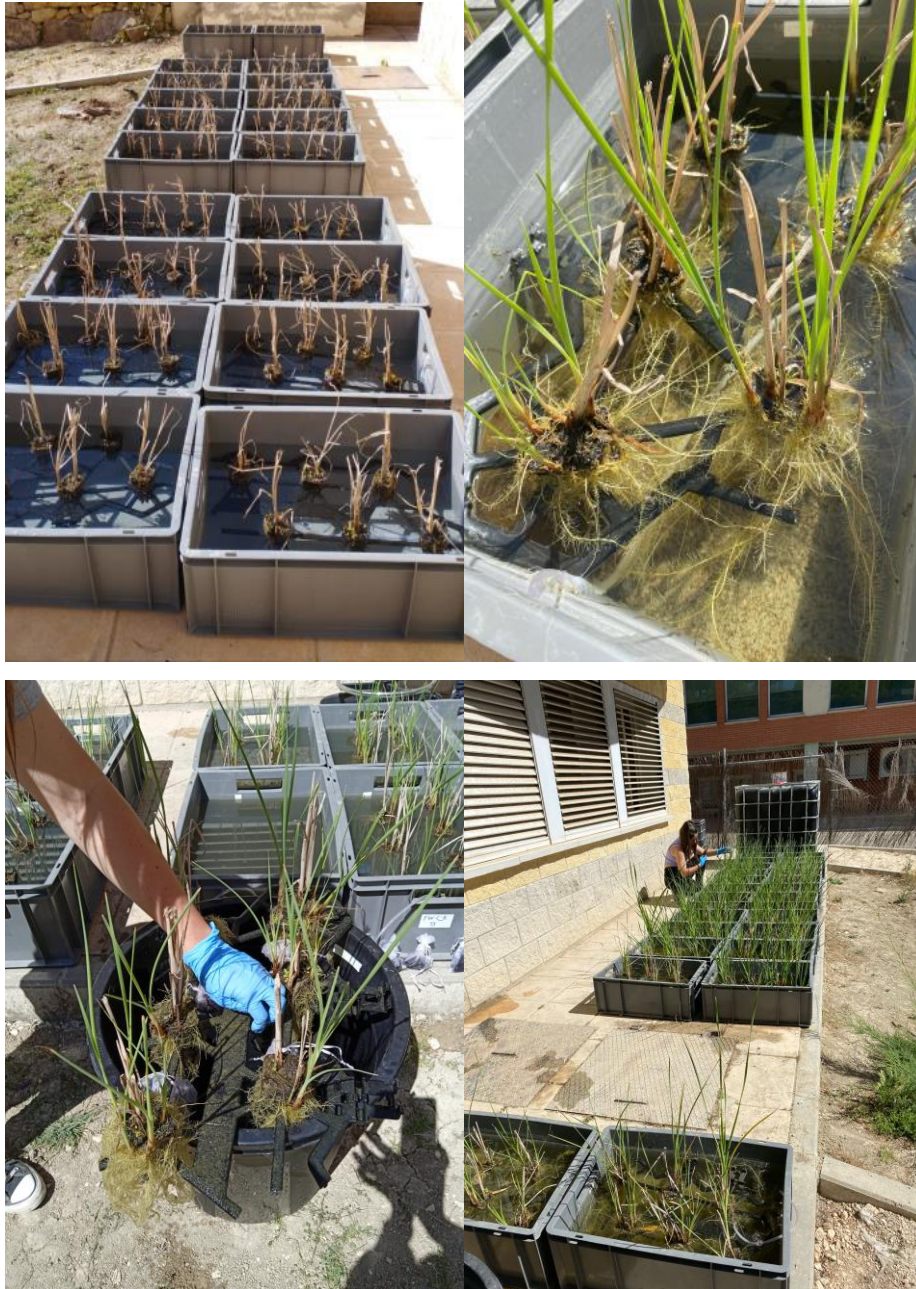
Fig S1. Microcosms with Floating wetlands, assembling 6 plants of Thypha sp. species in the plastic tile in each microcosm (following QUARQ ENTERPRISE S.A. instructions).
