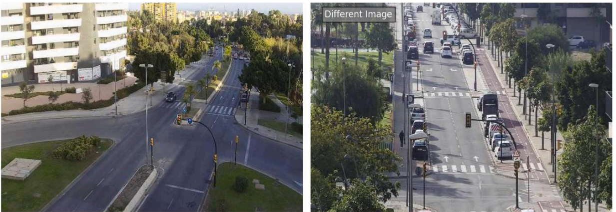
Fig. 5. Using a threshold M for common features, we determine whether the captured image corresponds to another location by comparing it to the reference image. This scenario occurs when the camera is pointed at a different location than usual to visualize a specific traffic event. Parking DISTRITO_10_TV63-JUANFRANCESBOSCA.
