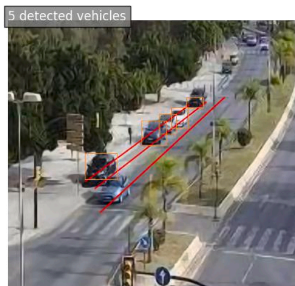
Fig. 8. Detecting the number of cars using YOLOv8x (confidence of 0.2) on a preprocessed image with OpenCV Super Resolution and Fast Non-Local Means Denoising (Colored) using an h parameter equal to 5. Parking DISTRITO_10_TV63-JUANFRANCESBOSCA.
