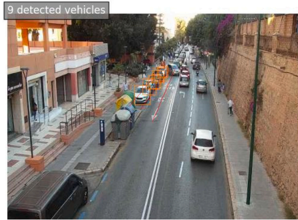
Fig. 9. An example of detecting multiple duplicate cars using YOLOv8x with a confidence threshold of 0.01. The intersection of these rectangles with the parking area boundary will be used to calculate the available parking spaces.
