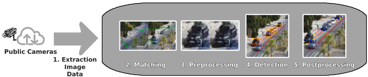
Fig. 1. The proposed pipeline consists of five main stages: Extraction, Matching, Preprocessing, Detection, and Postprocessing.
