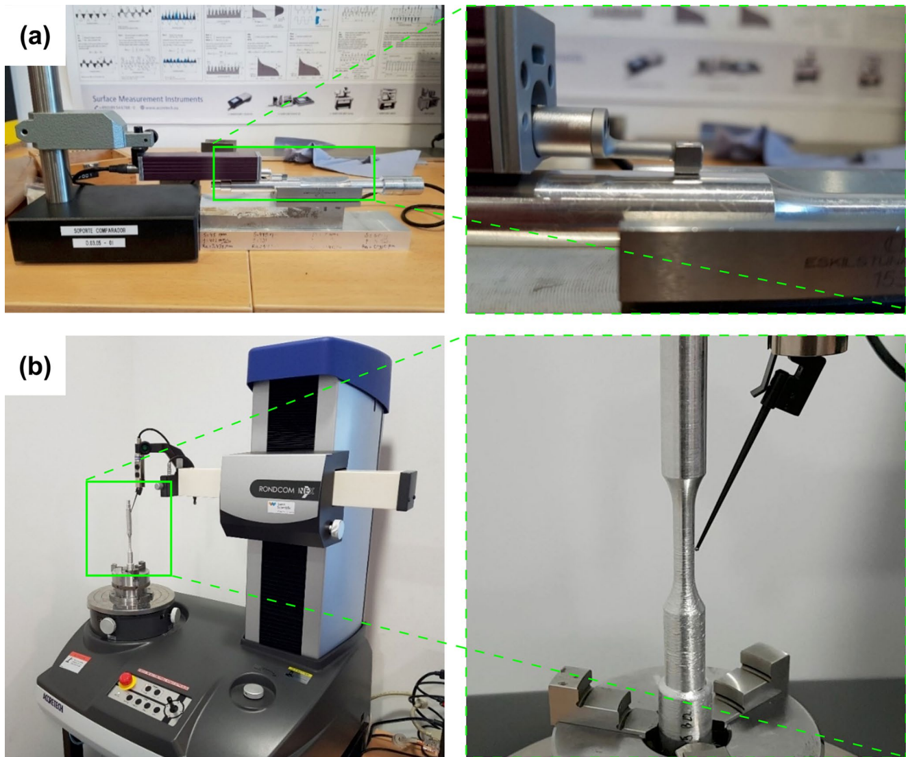
Fig. 3 (a) Surface roughness measurement; (b) measurement of form deviations
