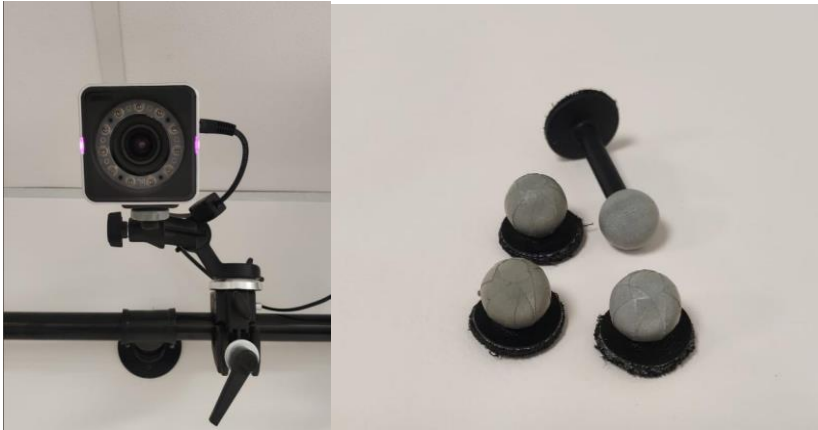
Figure 9. Infrared camera and reflective markers (Image created by the author).
