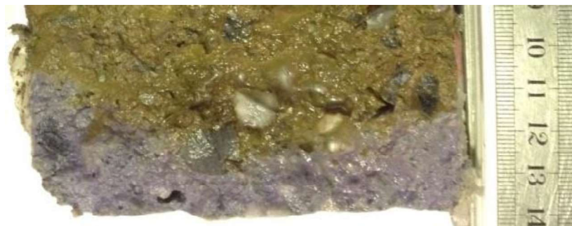
305 Figure 11. EA-10 concrete samples sprayed with 0.1 M AgNO 3 solution at 28 days.
