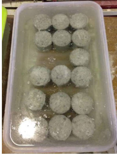
179 Figure 5. Concrete samples immersed in NaCl solution.
