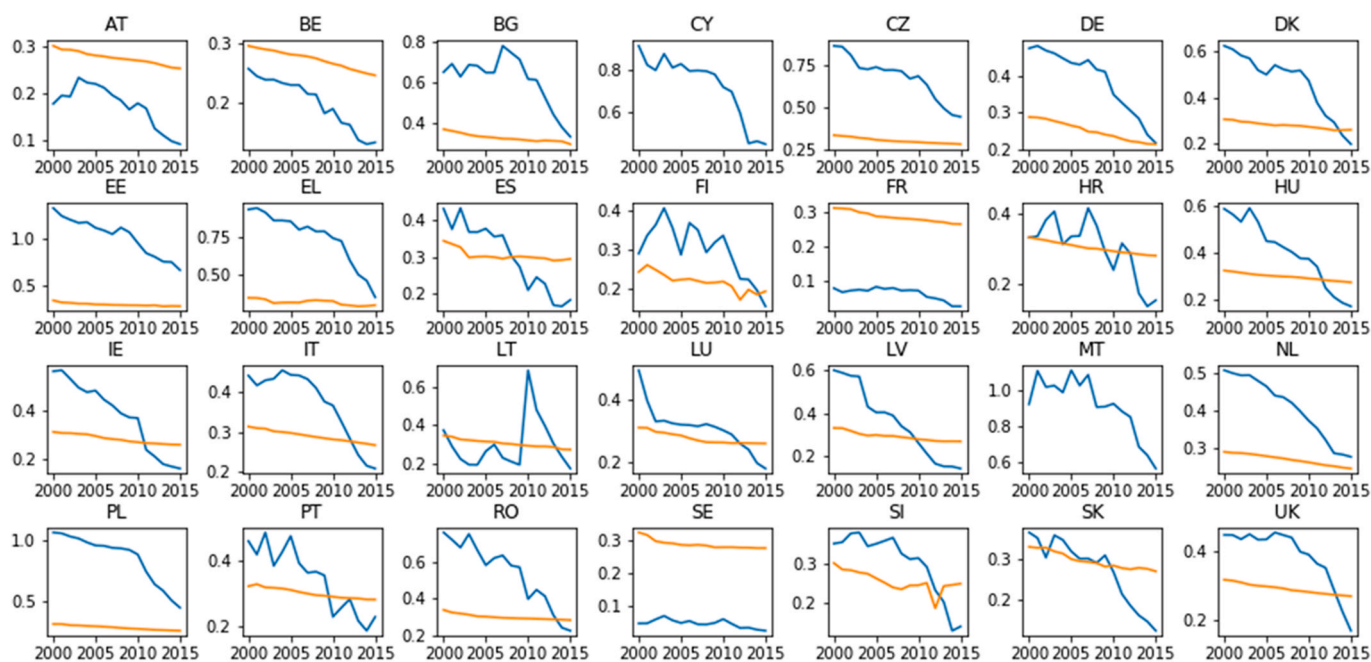
Fig. 6. Tons of CO 2 -emissions per MWh useful heat provided by heat pumps (blue) in comparison to conventional gas boilers (orange) for reference. Note that Cyprus and Malta do not have a gas network. Data source: JRC IDEES Database, Tertiary sector (JRC, 2018). (For interpretation of the references to colour in this figure legend, the reader is referred to the Web version of this article.)
