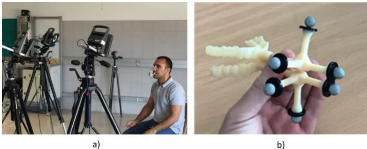
Figure 1.-a) Vicom infrared camera system. b) Trihedrons with markers to record mandible movements.
