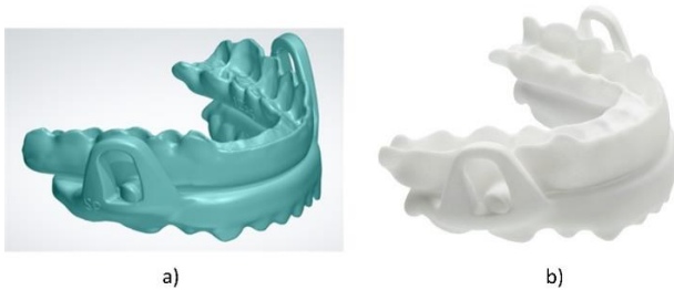
Figure 10.-Final design of MAD. a) CAD/CAM model device. b) Real device printed in 3D®.
