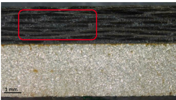
Fig. 11. Remains of the thermoplastic matrix adhering to the surface after machining that worsen surface quality.
