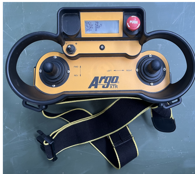
Figura 2.8: Control remoto de Hetronic .
